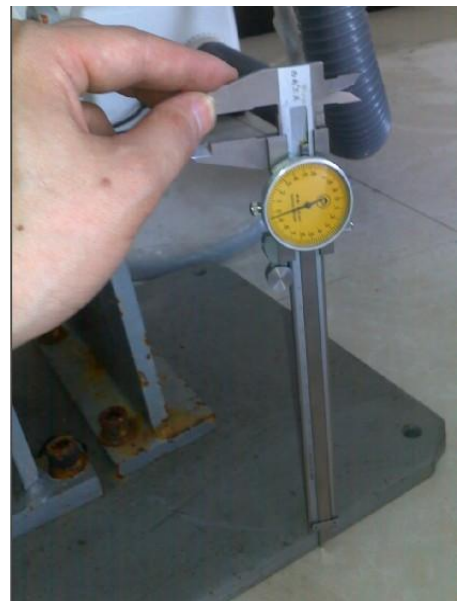
the steel thickness is 11.5mm
