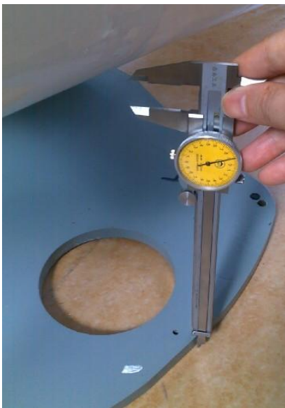
hongke steel thickness is 15.9 mm
